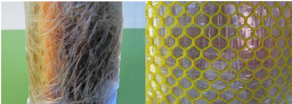
Before the use of ARMOR products, control rods were dipped in oil and wrapped (as pictured on the left). Now, vital pieces of the nuclear reactor such as the control rod (pictured right), are protected by ARMOR.
