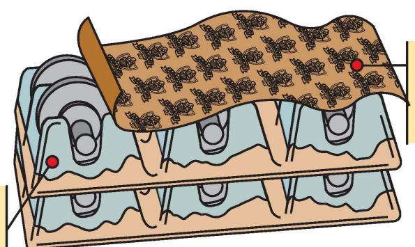
For best protection place ARMOR WRAP® VCI Paper or ARMOR POLY® VCI HDPE Film on top of parts
