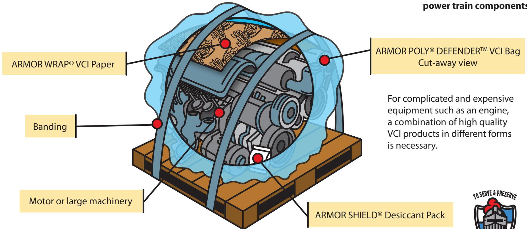
For complicated and expensive equipment such as an engine, a combination of high quality VCI products in different forms is necessary.
