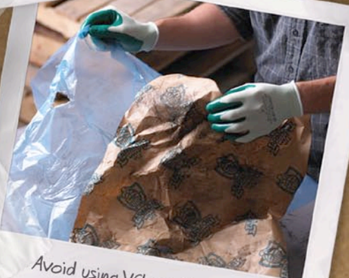
Use gloves when handling parts to eliminate rust caused by fingerprints.
