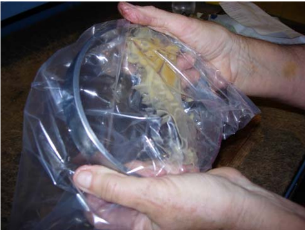
Moving part around oil to fully coat part
