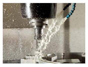
Metalworking fluids are represented by a wide variety of liquids used in the processes associated with reshaping metal objects into a desired form. They have evolved significantly over time to enhance particular performance characteristics and to alleviate health, safety and environmental concerns.
