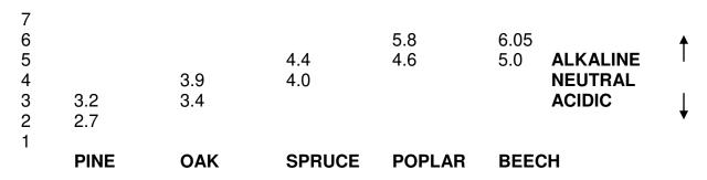
Overall, pine and oak are very acidic and can contribute greatly to corrosion issues. Avoid contact of metal with woods, especially pine and oak. By placing ARMOR WRAP® VCI Paper or ARMOR POLY® between these materials (or ARMOR SHIELD® VCI Corrugated or Chipboard) it will eliminate the contact corrosion and protect the metals from rust.
